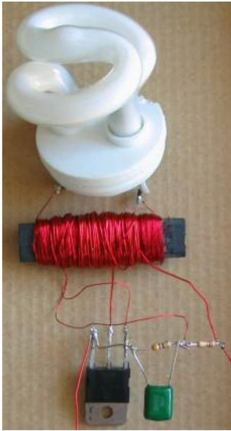
This circuit will drive a 5watt CFL tube from an old CFL lamp from 6v or 12v. It makes a very handy emergency light.
