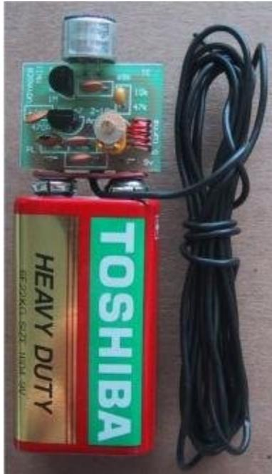
All the elements of good design have been achieved in this project. The circuit has a slightly higher output than the 3v circuit above, but most of the voltage is lost across the emitter resistor and not converted to RF. The main advantage of this design is being able to connect to a 9v battery. In a technical sense, about half the energy is wasted as the stages actually require about 4v - 5v for maximum output.
