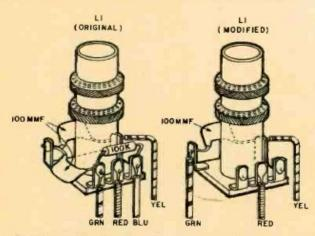
Coil L1 as it appears when removed from can, at left. Modify it by removing 100 mmi capacitor, 100 K resistor, blue lead; also move the green lead.
