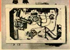
There's plenty of room for all parts in the chassis we selected. All leads should be short and direct to keep hum and distortion low and to assure proper oscillator (V2) operation. Braid on shielded lead from J2 to R5 is grounded at J2 only. Twist AC lead to S1 and position it near the chassis.
