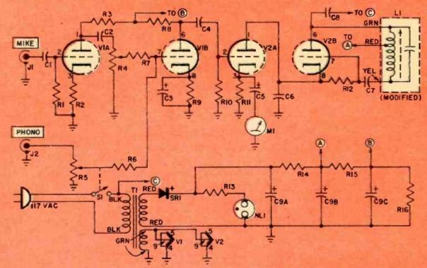
Mike signal is amplified by VIA and fed via R4 to VIB and further amplified. The signal continues to V2A which, because it is connected between Hartley oscillator V2B and ground, modulates the oscillator.
