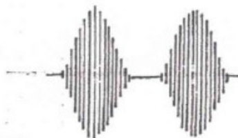
Fig. 6 E 150 % modulation (tone) (without carrier-control)
